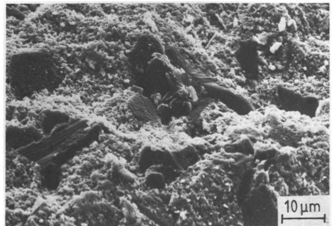
Fig. 10. Fracture surface of 2Y-TZP containing 10 vol% \text{Al}_2\text{O}_3 platelets.
